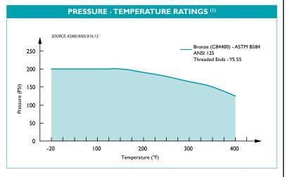
1. The pressure-temperature ratings given are ONLY for the YS 55-BZ (Threaded) per ASME B16.15. The internal working pressure rating for a solder joint strainer is dependent, not only on the strainer, but also on the composition of the solder used for the joint. The working pressure ratings shown for model YS 56-BZ (Solder) are representative of using an alloy Sb5 95-5 tin-antimony solder. For other solder joints, please consult factory.
