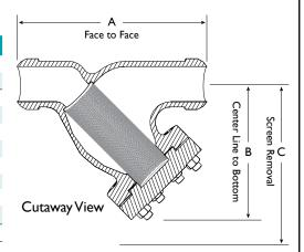
**ASME Class 900 Butt Welded ends have a schedule of 160.** Illustrations are representative of sizes 2" through 10". Please ask for certified drawings when required.
