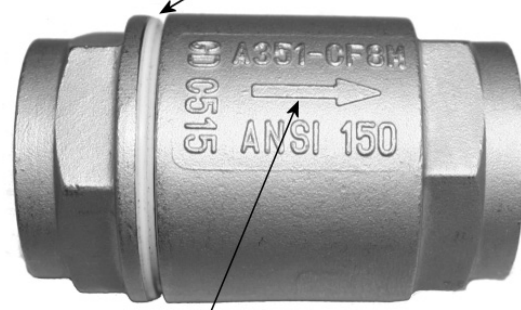
Figure 5: CV 80-SS showing unwanted gaps between the two body pieces
