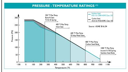
The above chart displays the pressure-temperature ratings for the valve's body material per ASME B16.34. Max temperature limits have been added for seat and spring materials.
