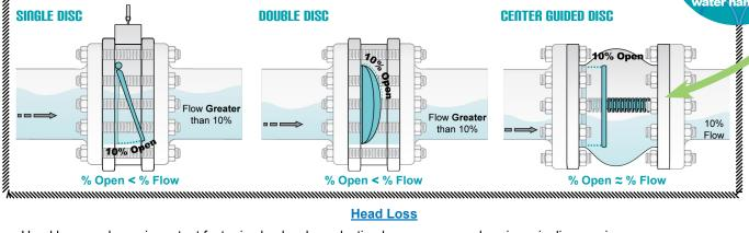
Head loss can be an important factor in check valve selection because energy loss in a pipeline can increase expenses significantly over time in certain applications. The main design features that affect head loss are the internal shape of the body and obstructions to the flow. Titan's Check Valves are designed with the following features to minimize head loss:
