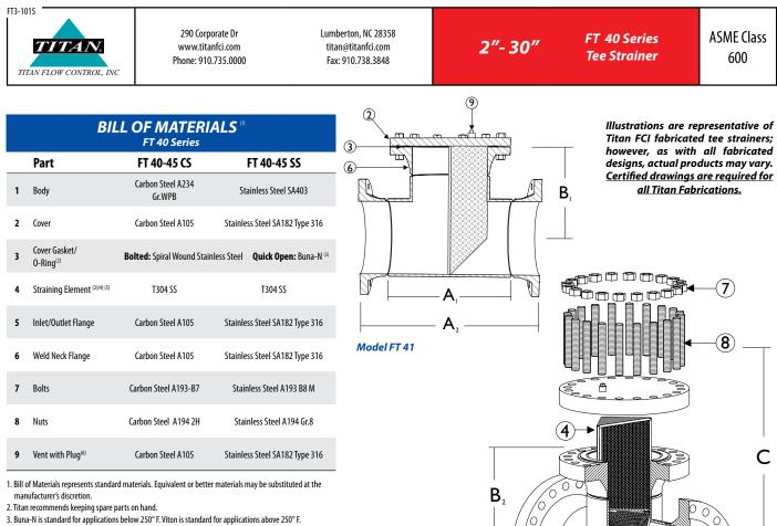
3. Buna-N is standard for applications below 250° F. Viton is standard for applications above 250° F.
