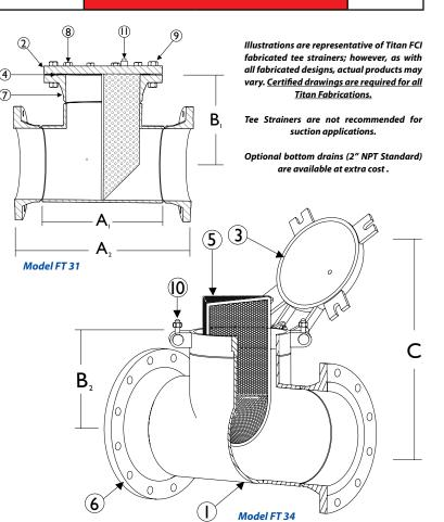
Buna-N is standard for applications below 250° F. Viton is standard for applications above 250° F.
