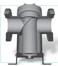
**BASKET STRAINERS** are used commonly in horizontal applications where cleaning will be less frequent. Because of their larger bodies, they typically provide more open area for debris collection than Y-strainers. The straining element (a.k.a the "basket") for a basket strainer has a handle for easy removal and secure placement within the strainer's body. The basket can have a slanted top design (as shown to the left) or a straight top design.
